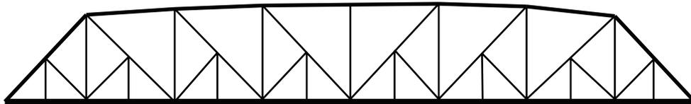
**2.1** How many triangles of any size are there in the Pennsylvania truss bridge shown?
